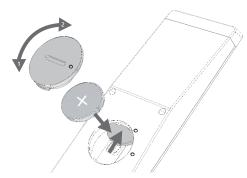
Twist the battery compartment lid out in an anti-clockwise direction and then remove it. Insert a CR2032/DL2032 battery. The plus pole of the battery must point upwards here. Replace the battery compartment cover onto the remote control (observe the markings).
