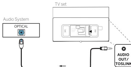
Connect the audio output of the TV labelled AUDIO OUT TOSLINK to the digital audio input of an audio system.
