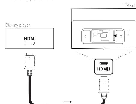
Connect the device by an HDMI cable with a Type A connector (not supplied) to one of the HDMI sockets of the TV set. To fully enjoy the capabilities of your TV, use a cable labelled „Premium High-Speed HDMI Cable“ or better.
