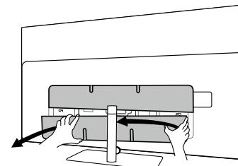
When connecting external devices to these internal connectors, first connect the cable to the connector on the TV set. Then route the cable out of the TV using the built-in cable management system, and then route the cable through the neck of the stand (in case you use provided Table stand solution).
