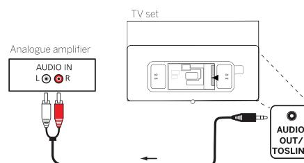
Use a stereo cinch/jack adaptor cable to connect the audio output AUDIO OUT TOSLINK to the analogue audio input of the audio system.
