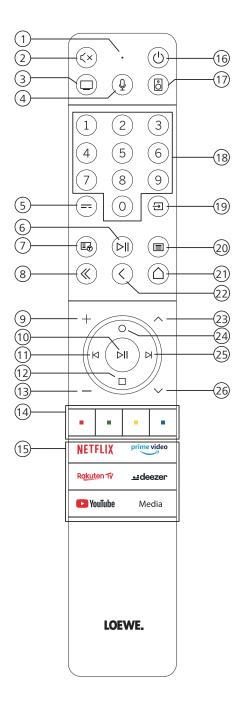
You can connect your remote control to the Loewe TV via Bluetooth standard. To do this, press and hold the Menu button 20 for at least three seconds. Observe the screen displays for successful pairing.
