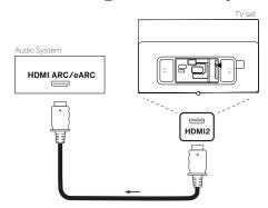
Use an HDMI cable (not supplied) to connect HDMI eARC socket of the TV set to the HDMI ARC/eARC socket of an audio system or soundbar. It is recommended to use a cable marked as "Ultra High-Speed HDMI Cable" with a Type A connector.
