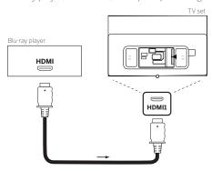
Connect the device by an HDMI cable with a Type A connector (not supplied) to one of the HDMI sockets of the TV set. To fully enjoy the capabilities of your TV, use a cable labelled "Premium High-Speed HDMI Cable" or better.
