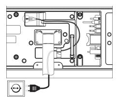
Connect the mains supply plug of the mains supply cable to a power outlet.
